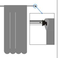
4 Attach each Hook End of the Drape Support to the top of the Upright.
